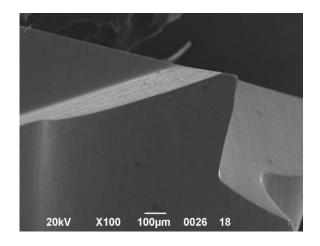
The samples of group 1 showed surfaces particularly altered after the standard cleaning treatment. In the craniotome case on the surface it were identified some particles whose total area represented 4.19% of the total area of the craniotome itself; these particles have a uniform chemical composition: calcium, phosphorus, oxygen (bone tissue residue) and other trace elements, these data were obtained by scanning electron microscope (SEM) analysis.
