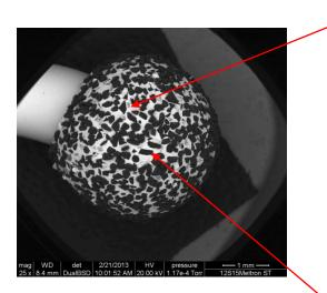
PARTICLES MICROANALYSIS: main elements found are NICKEL (upper spectrum) and CARBON (lower spectrum)
