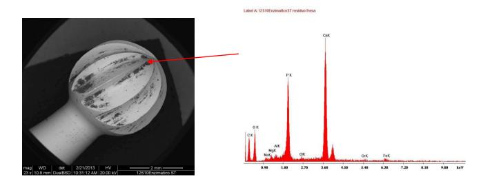
DARK PARTICLE MICROANALYSIS: main elements found are CALCIUM, PHOSPHORUS, OXYGEN (bone tissue residue)
