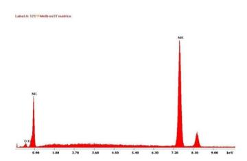
MATRIX MICROANALYSIS: main element found is NICKEL (upper spectrum)
