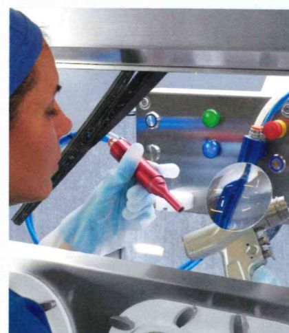
Fig. 1: The mechanical action is ensured by the impact of sodium bicarbonate molecules with a calibrated granulometry (400 microns) and will allow the elimination of stains without causing abrasion of the surface of stainless instruments.
